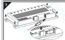
Install the Control Box properly with the included screws.
