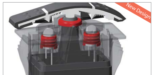
Advanced water-tight sealing design (Patented)
