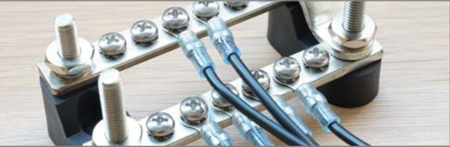
Bus height differentials allow cable output from the same side (BF427)
